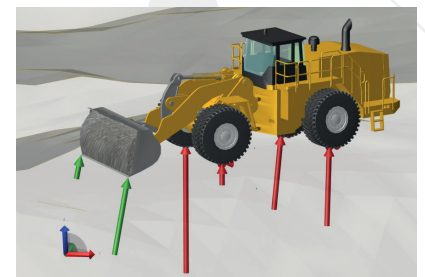
Simulation of a wheel loader: Visualization of the forces on wheels and bucket in SimulationX
